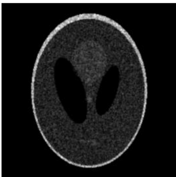
Fig. 3 The filtered image, where a nonstationary filter is applied with a=0.175 , b=0.01 and c=0.6 in Eq. (3). The RMSE is 0.6010
