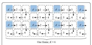
Fig. 1 Formation of the frame by the RCDOER-matrix
